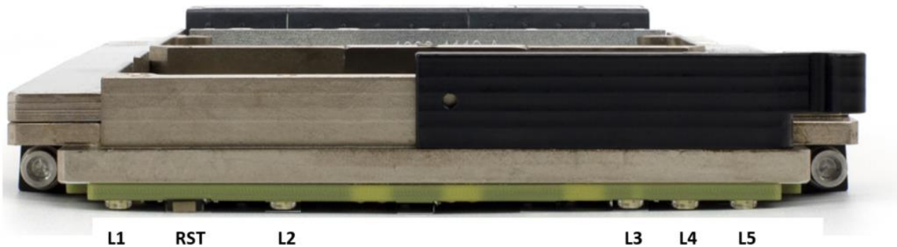
Figure 6: RC variant - Front Panel with LED indicators and reset button (front view of an ECL 3xxxxyy board)
