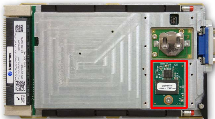
Figure 50: Mezzanine Slots Location
