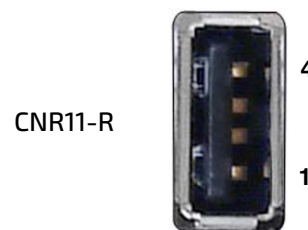
Figure 37: Front Panel USB Connector
