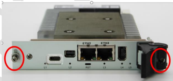
Figure 12: Air Cooled variant - Screws Location on the front panel
