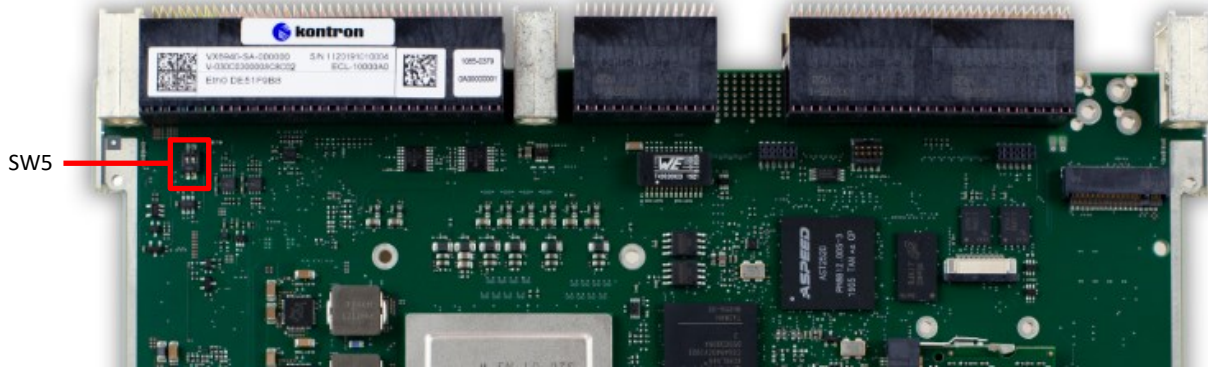
Figure 16: VX6940 Board Configuration - Microswitches (Top side)
