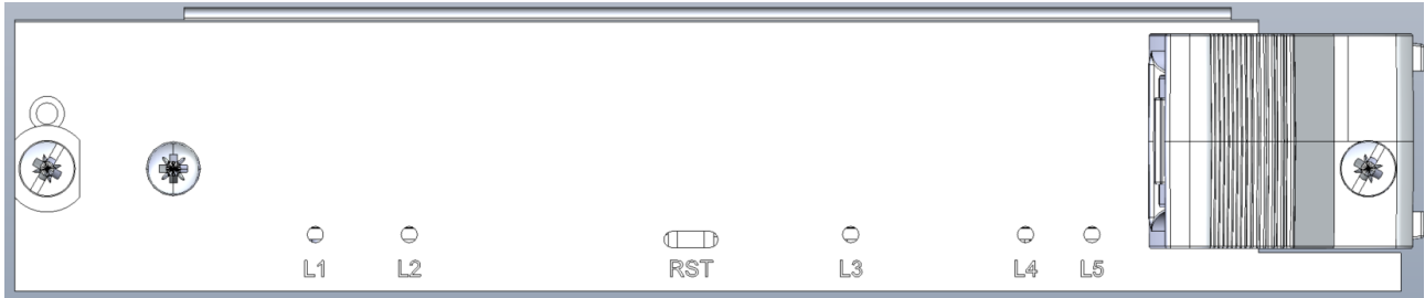
Figure 6: RC3 variant - Front Panel Interfaces - FB-VX3-0010 tooling option not equipped
