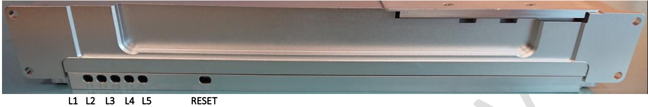
Figure 10: RC variant - Front Panel with LED indicators and reset button
