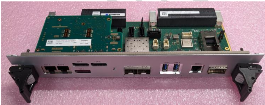
Figure 41: RTM with the optional PIM-VX-2DP-WOLF module installed
