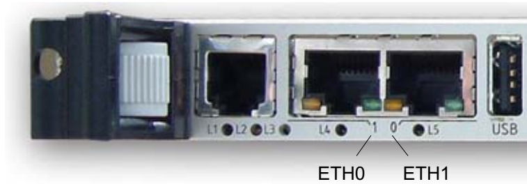
Inversion of the numbering of the Ethernet connectors
