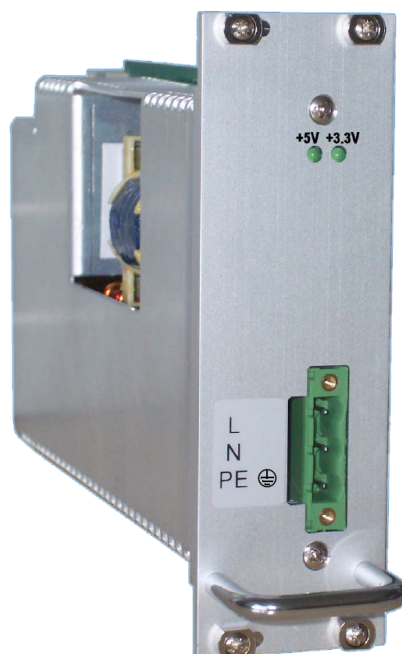
// View of Power Supply Unit CP3-SVE-M76AC-230
