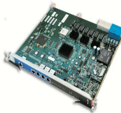
AT8900 Ethernet switch
