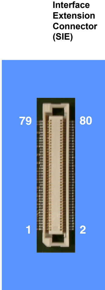
Figure 2-7: J22 - System Interface Extension Connector (SIE) Table 2-11: Pinout of J22 (P2) Connector
