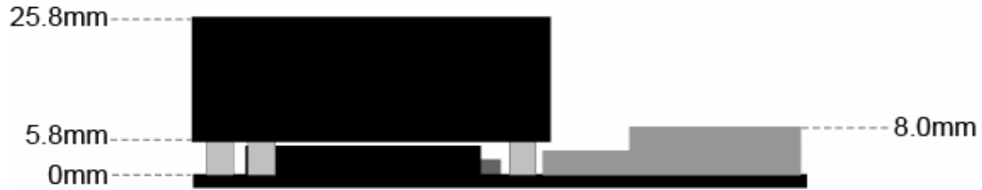
Figure 8: 2nd Side View with Heat Spreader
