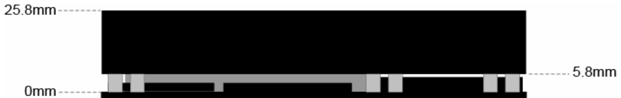
Figure 7: Side View with Heat Spreader
