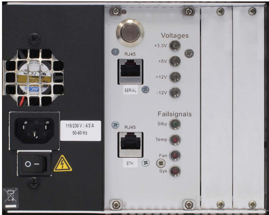
Figure 8 : LEDs Overview on EZ3-CMB Rear Panel
