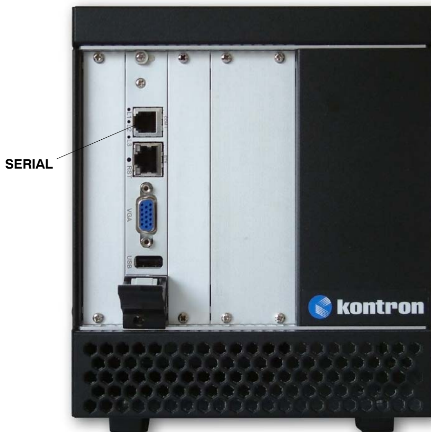
Figure 11: Linux Pre-Installed System Parameters: Serial Line / Console Output
