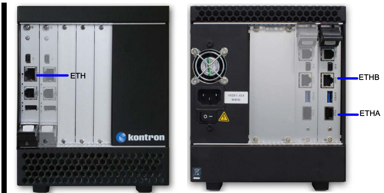
Figure 8: Hardware Name of Ethernet Ports
