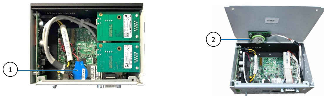
Figure 12: RTC Lithium Battery Installed
