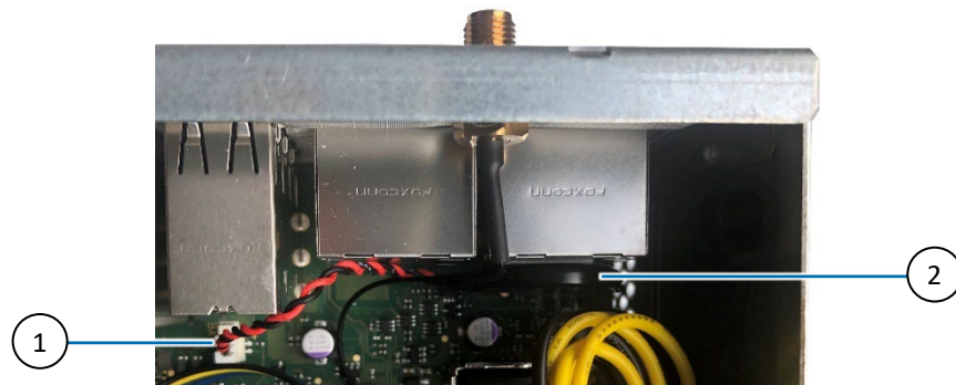
Figure 24: CR2032 Lithium Battery and BAT header
