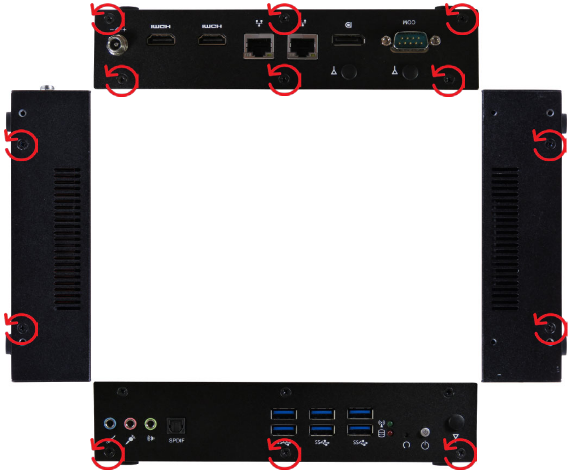
Figure 9: Descrewing two chassis halves of the KBox F-210 Series
