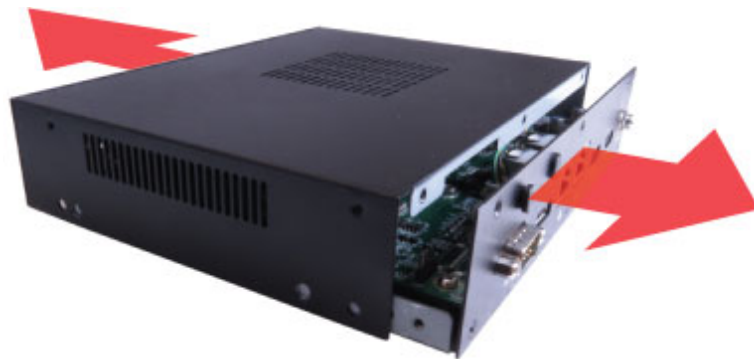
Figure 10: Disengaging the chassis of the KBox F-210 Series
