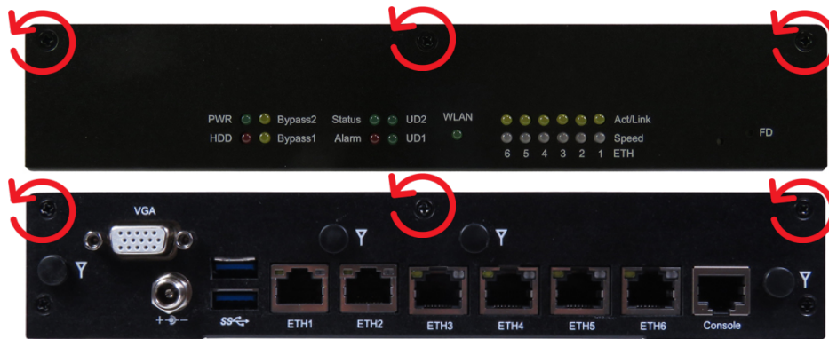
Figure 8: Descrewing the access cover of the KBox N-110 Series
