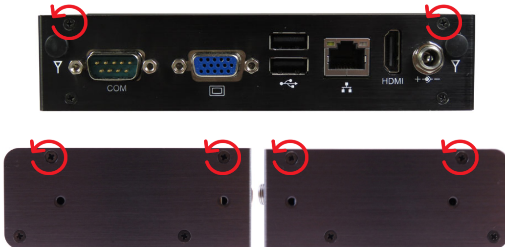
Figure 5: Descrewing the access cover of the KBox P-100 Series
