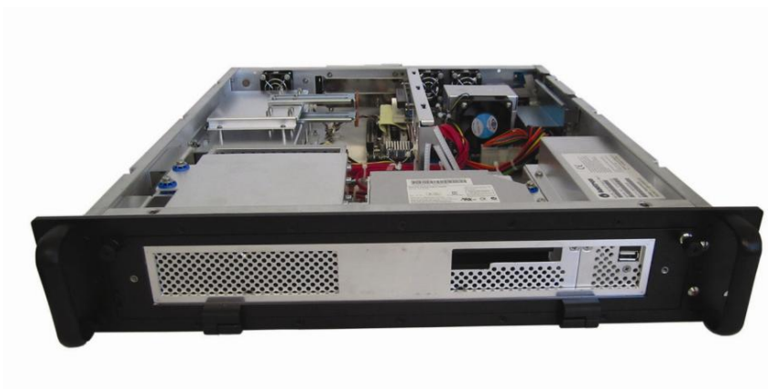
Fig. 20: Open to show Front Screw Fixing Bracket
