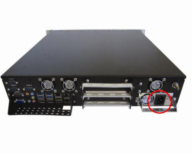
Fig. 27: Back of KISS Oil & Gas 2U showing power cable socket on the right side of the system
