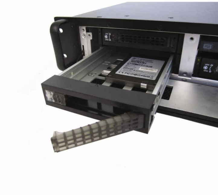
Fig. 23: Gently pull open drive bay and remove/replace the drive.
