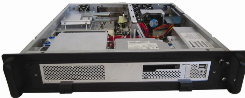
Fig. 6: View from the front of the KISS Oil & Gas 2U with the top panel and filter/ filter cover removed
