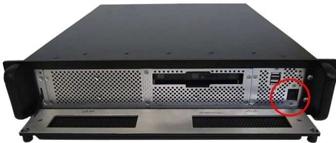
Fig. 27: Back of KISS Oil & Gas 2U showing power cable socket on the right side of the system
