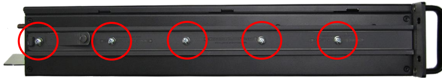
Fig. 35: Side system view: Attaching the inner section of the slide rails 5x M4x6 round headed screws for each side
