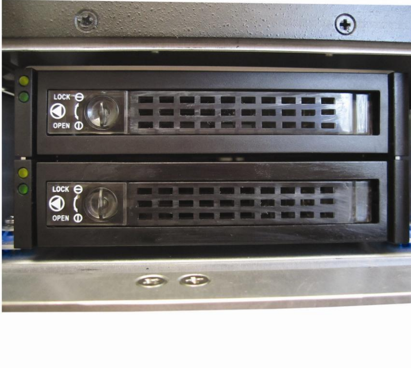
Fig. 22: 2 of the 3 removable drives behind the drive cover
