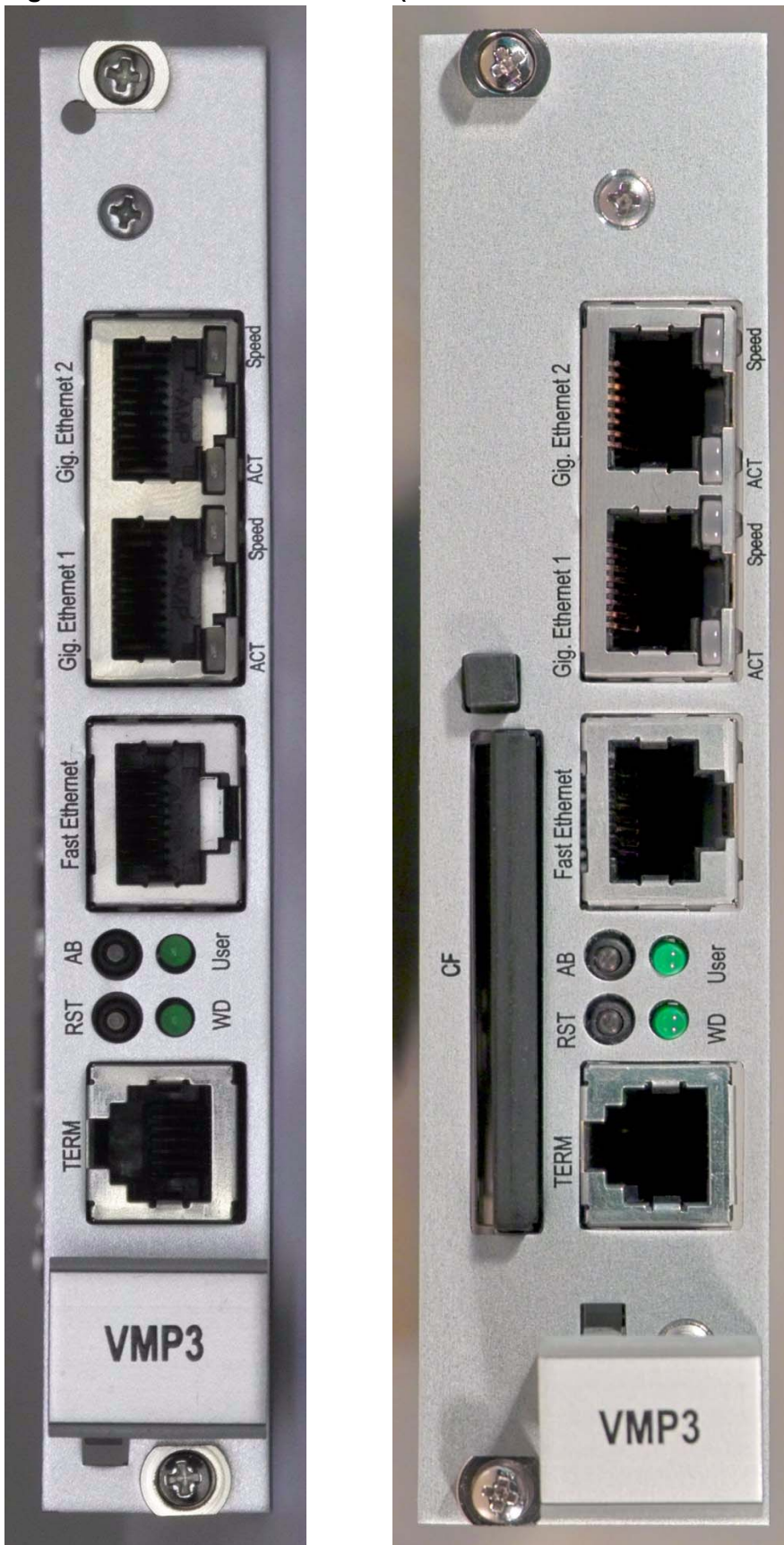
Figure 1-7: VMP3 Front Panels (4HP Standard and 6HP with CompactFlash)
