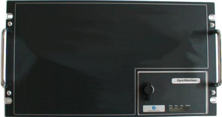
Fig. 4b: Front panel without LCD display, without membrane keyboard and without touchpad
