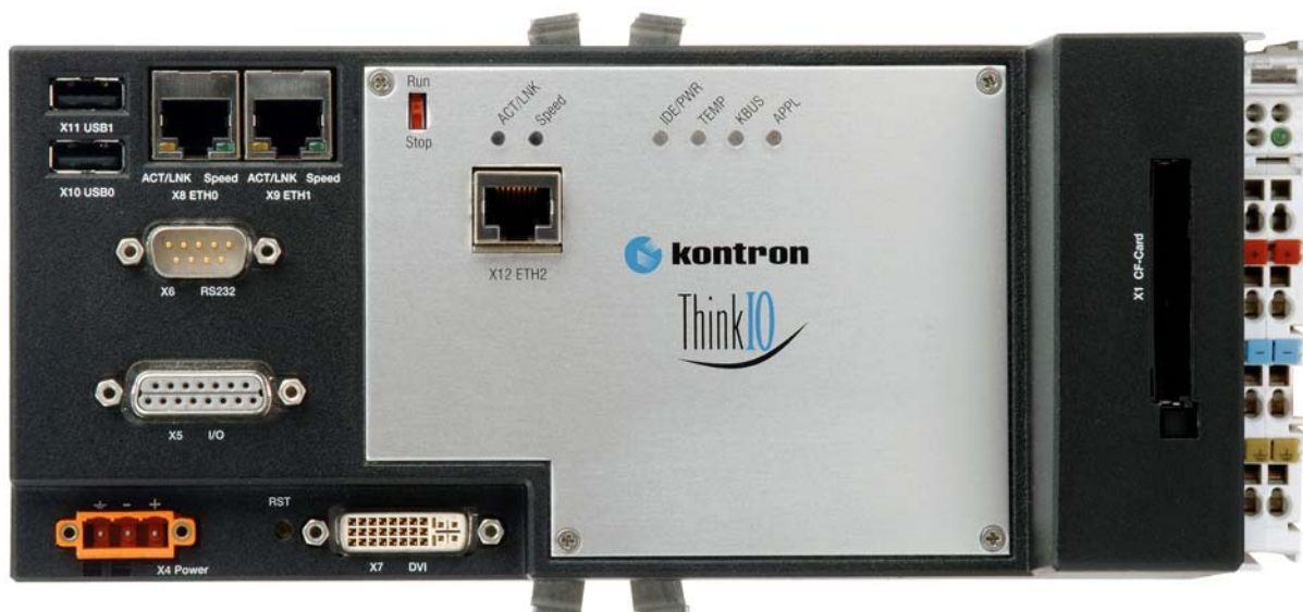
Figure 1: ThinkIO-Duo with the WAGO Interface Module (K-Bus) Assembled
