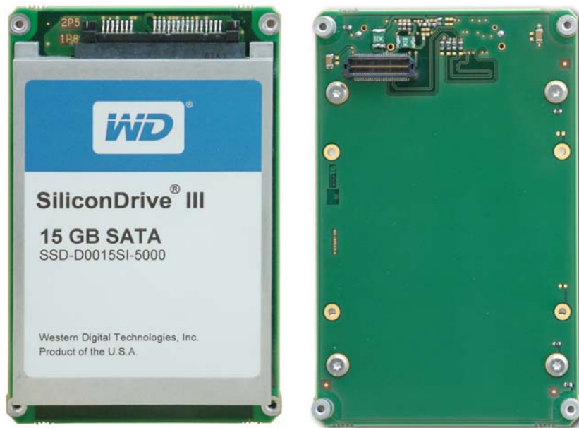
Figure 16: SATA Extension Module: front and Bottom Views
