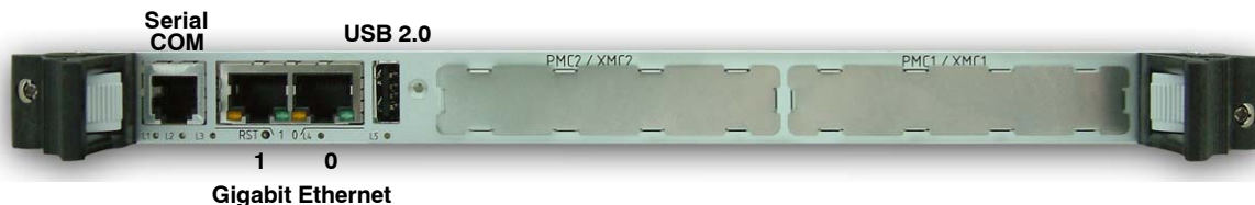
Figure 30: Location of the Front Panel Connectors
