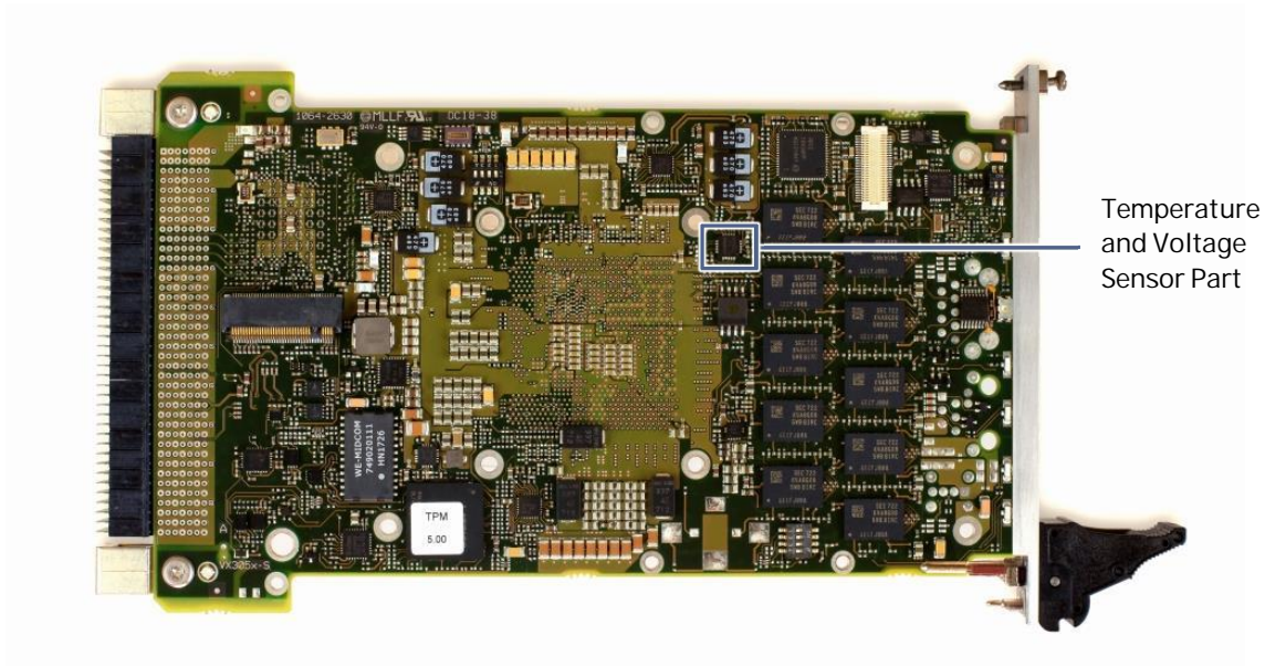
Figure 27: Temperature Sensor Location
