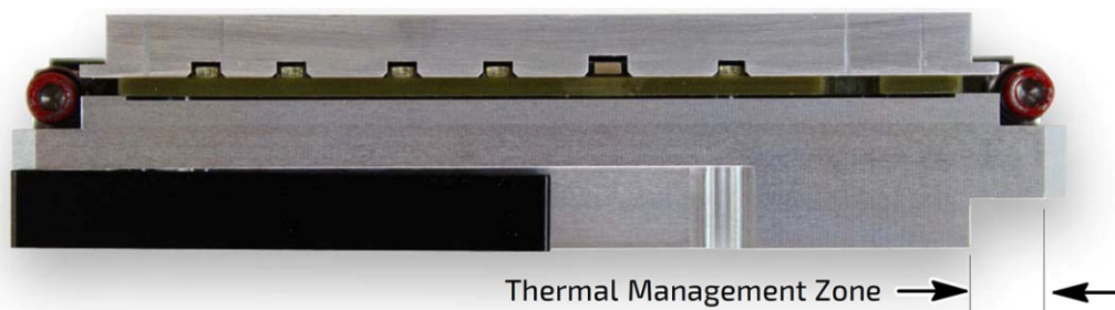
Figure 36: VX305x-RCThermal Management Zone
