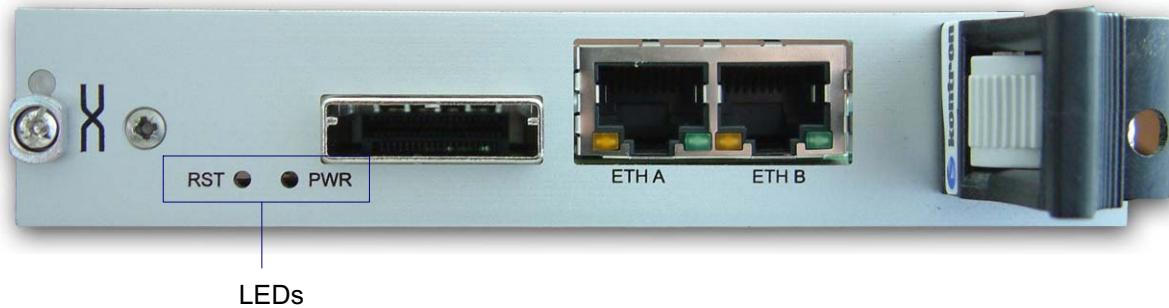
Figure 5: Front Panel Status LEDs of the VX3905
