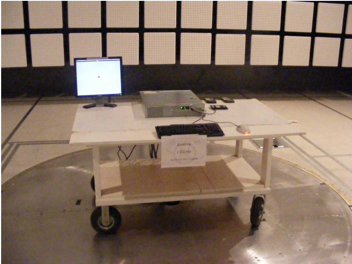
Photograph 4. Radiated Emissions Test Configuration
