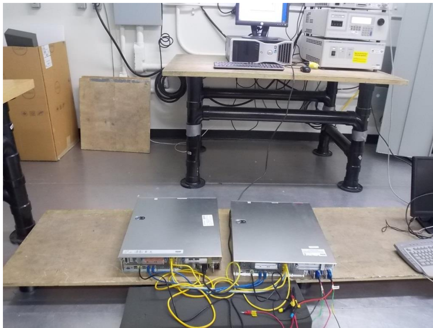
Figure 8.11-1: Voltage dips and voltage interruptions setup photo
