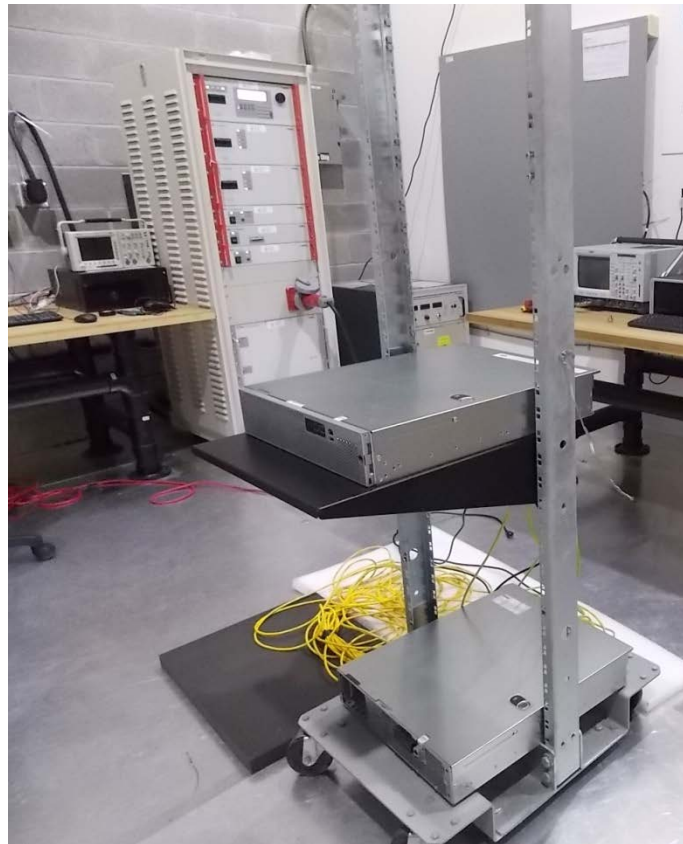
Figure 8.6-1: Voltage dips and voltage interruptions setup photo
