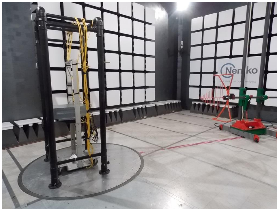
Figure 8.1-4: Radiated disturbance setup photo 30 to 1000 MHz
