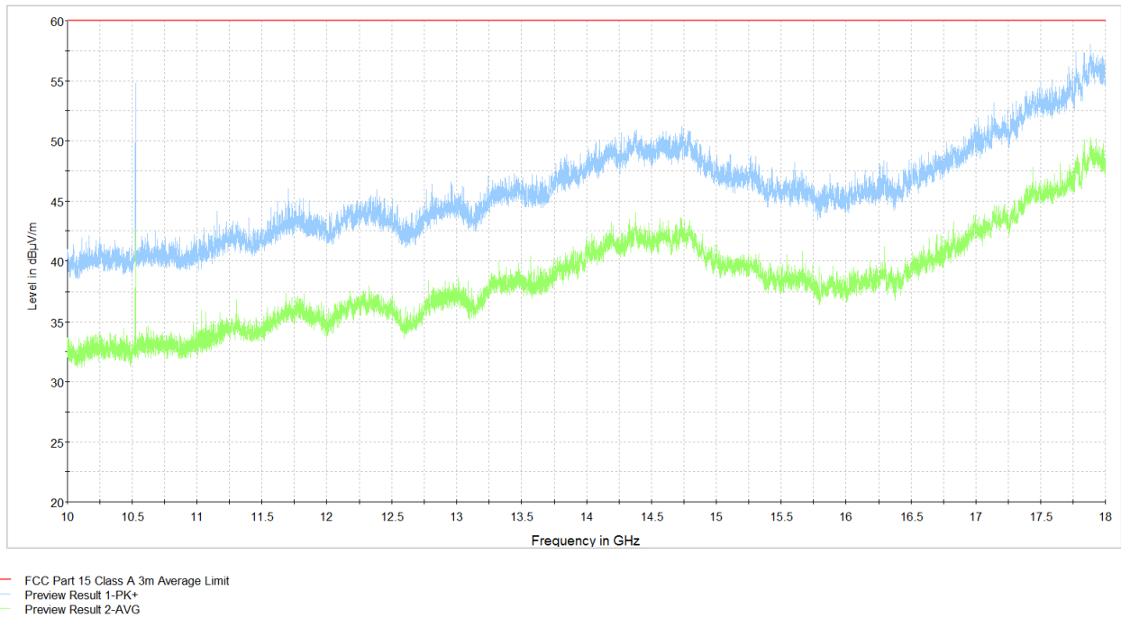
Figure 8.1-4: Radiated disturbance spectral plot (10 to 18 GHz)
