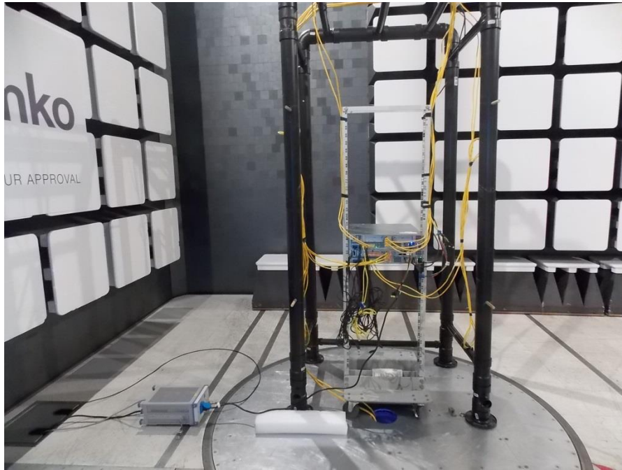
Figure 8.2-3: DC ports – Conducted emissions setup photo
