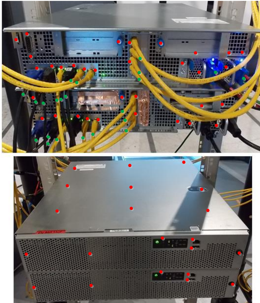
Figure 8.6-1: Electrostatic discharge test location point's photo
