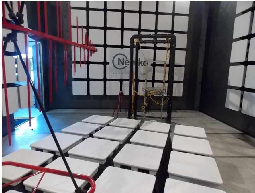
Figure 8.4-1: Radio frequency electromagnetic field amplitude modulated setup photo
