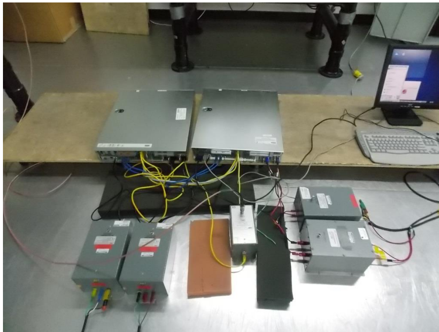
Figure 8.5-1: Radio frequency, conducted continuous setup photo
