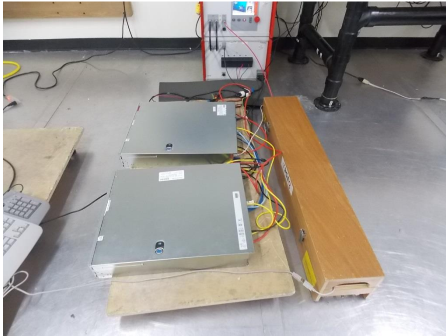
Figure 8.8-1: Fast transients setup photo
