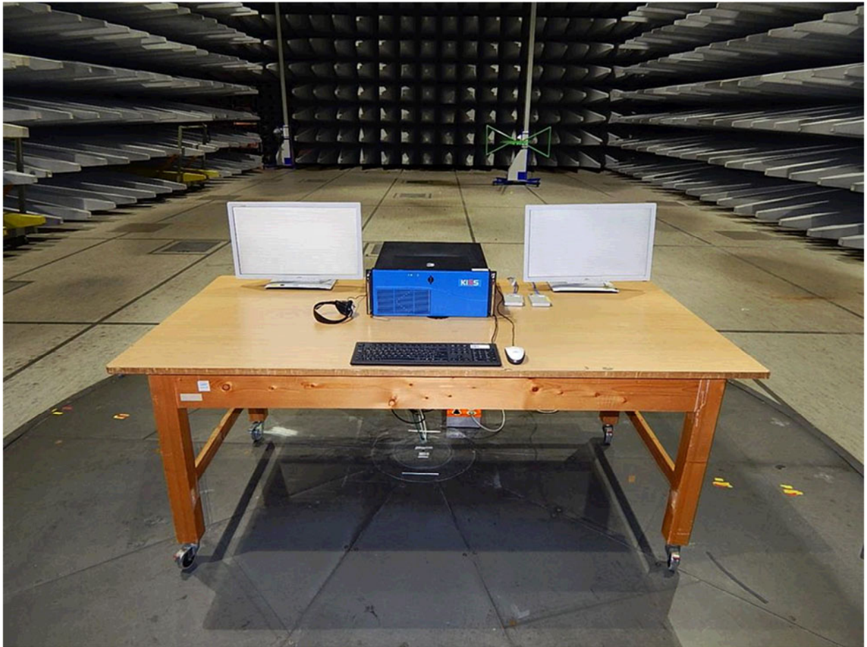
Figure 1 : Test set up Radiated Disturbance Emission - front view
