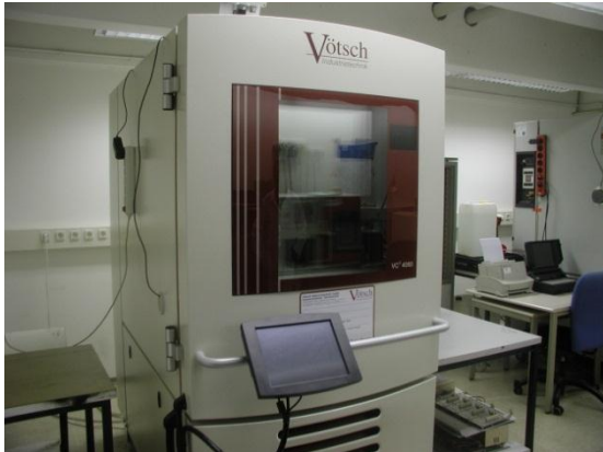
Fig. 10: Climatic chamber with control PC
