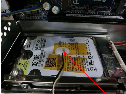
HDD (removeable) Sensor 5
